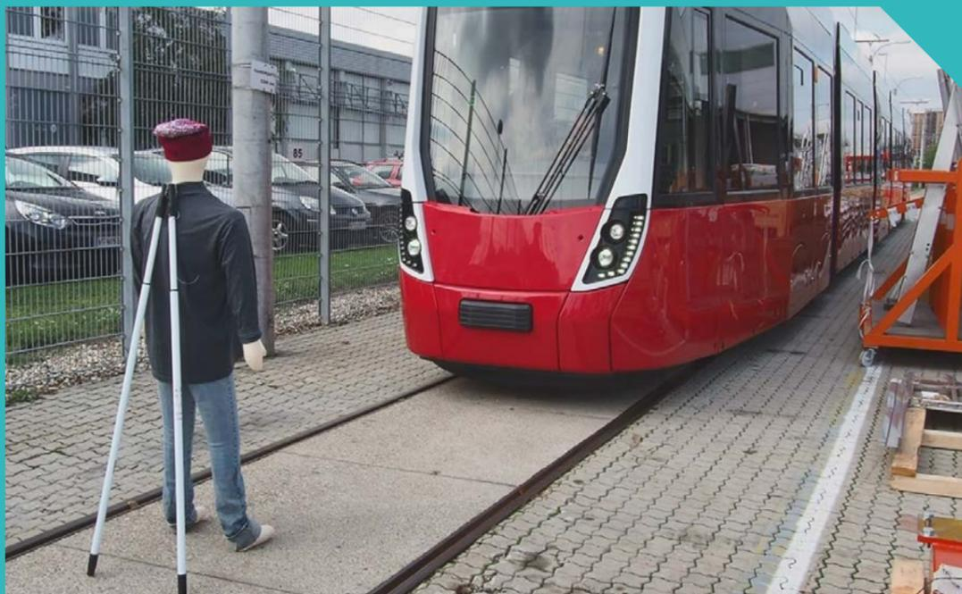
In case of danger the driver assistance system warns or stops automatically
