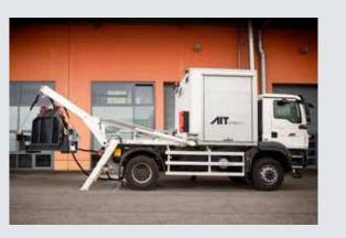
MoSeS: We use our Mobile Seismic Simulator (15-25 kN/1-80 Hz), a hydraulic vibration generator, to simulate vibrations or induce them in the ground and in buildings.
