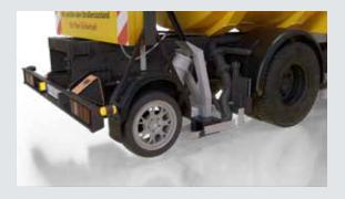
In order to measure skid resistance, we use an internationally standardized car tyre in the right wheel track. The friction force is put in relation to the tyre load and used to calculate a friction coefficient.
