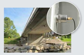
**Bridge monitoring:** Permanently-installed sensors allow us to continuously record data and transmit it, automate data evaluation and measurement report creation, and send warnings in case of exceeded limits.
