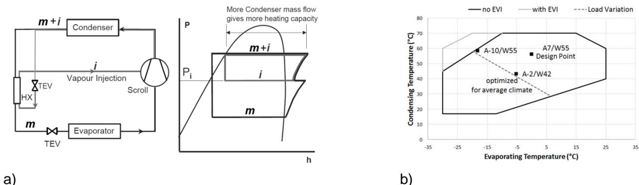
Figure 19: a) Scheme of the EVI-Cycle (Bella 2015). b) Operating range with/without EVI (Emerson 2015).
