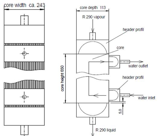
Figure 21: Drawing of single MPE tube, (B. Nitsch, AKG)
