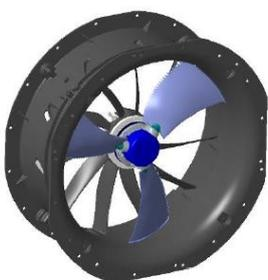
**Figure 41: Best fan geometry in CAD view (Ziehl-Abegg)**
