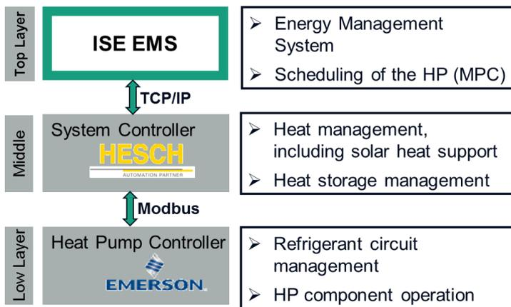
The controller hierarchy depicted in Figure 11 consists of three levels (layers):
