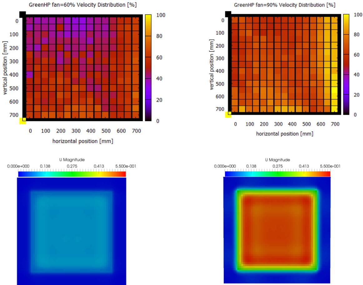
**Figure 37: a) Velocity distribution [m/s] under heat exchanger, fan 60% b) and 90%, experiments (above) and simulations (below) in the suction mode (the velocity scale for the two modes kept the same).**
