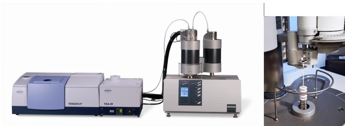
Fig. 26: Microbalance with simultaneous DTA, DSC, EGA (QMS, FTIR). Right: STA-DSC sensor of STA 449 F5 with automatized sample changer
