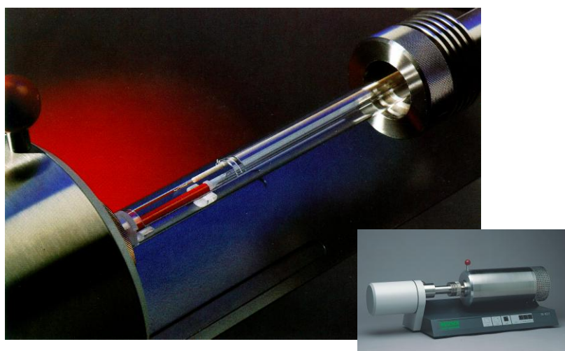
Fig. 2: Push rod dilatometer with sample carrier, push rod and sample (red)
