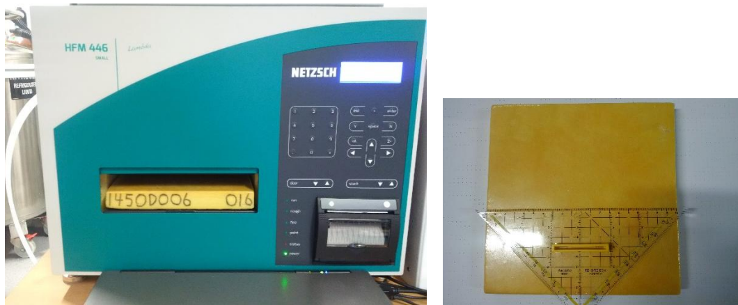
Fig. 23: HFM device NETZSCH HFM 466 Lambda with reference specimen (right, representing typical size of specimen)
