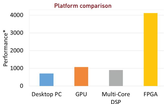
\*) Million disparity evaluations per second. Test - image size 450x375 pixels, 60 disparities. Desktop PC: Intel i7 with 4x2 Cores and 3GHz; GPU: GTX280 with 240 Cores and 1.3GHz; Multi-Core DSP: TMS320C6678 with 8 Cores and 1GHz; FPGA: XC7Z020 with 150MHz.
