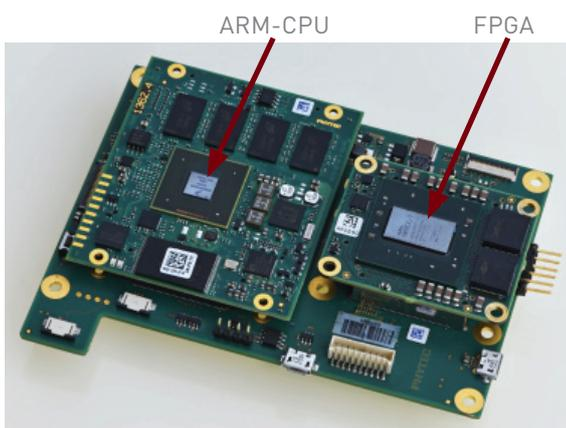
FPGA calculates high quality depth images in real-time
