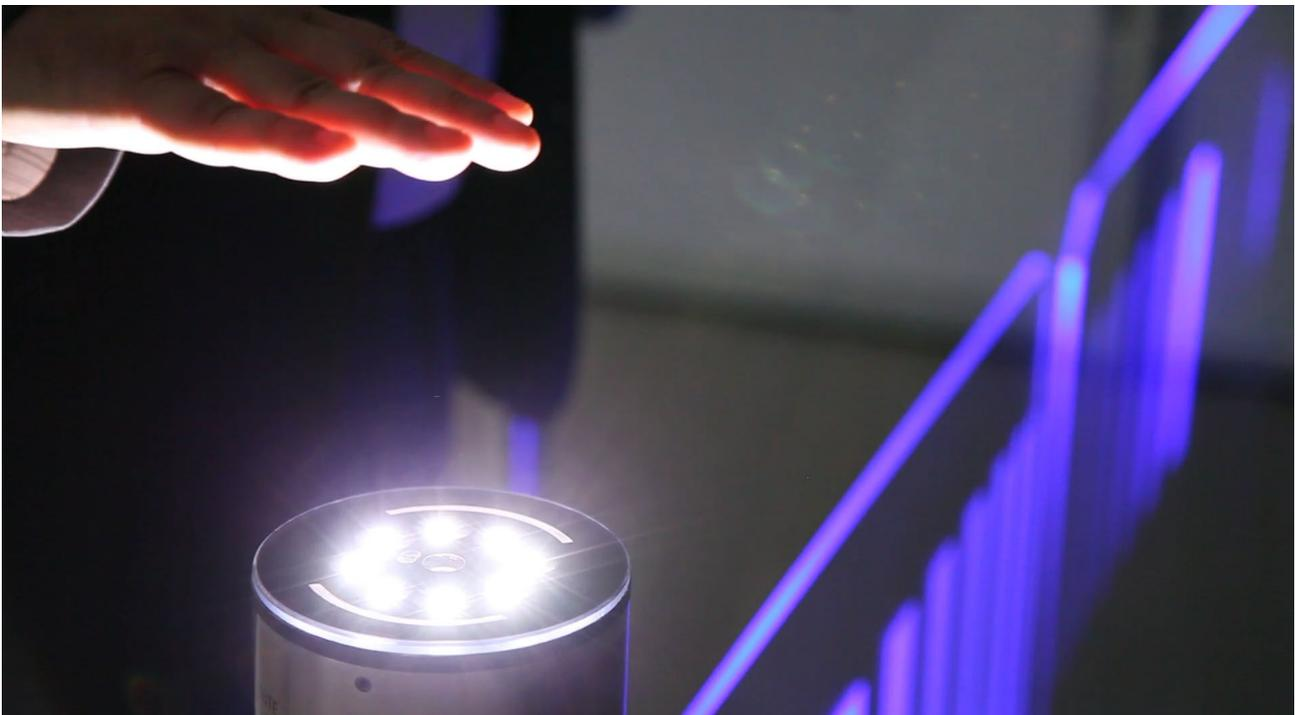
*Figure: contactless fingerprints scanner integrated in eGate*
