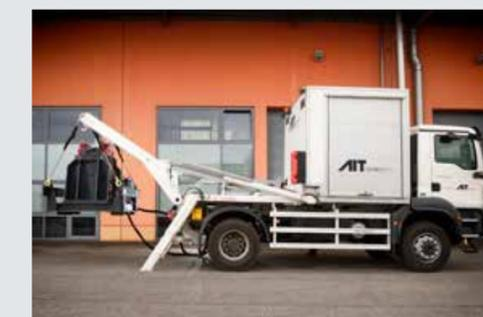
**MoSeS:** We use our Mobile Seismic Simulator (15-25 kN/1-80 Hz), a hydraulic vibration generator, to simulate vibrations or induce them in the ground and in buildings.
