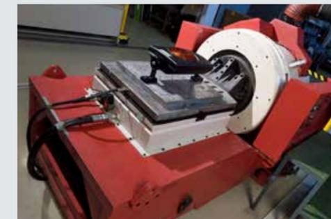
As an accredited testing laboratory for shock and vibration tests, we use our electrodynamic shaker to conduct tests for electronic and electrical components, devices, machines, systems and superstructures for vehicle parts – optionally using a climatic chamber.
