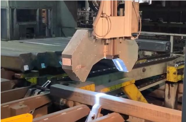
Photo credit: AIT Caption: The AIT inspection system during the inspection of a so-called rolling billet made of steel.
