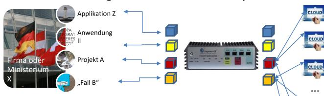
The credentials required for each S3 "location" are stored on a hardware-protected USB security stick. Every fragmentiX box is "stateless" without these USB sticks, it does not store any data statically.
