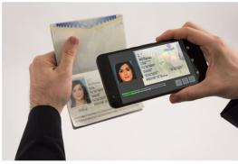
Figure: MRZ reading of a passport
