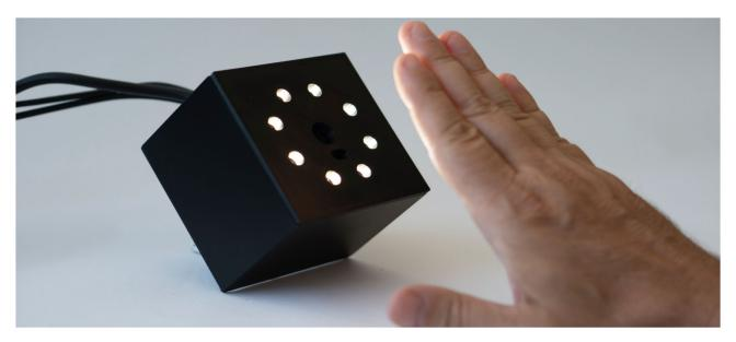
Figure: contactless fingerprint sensor system
