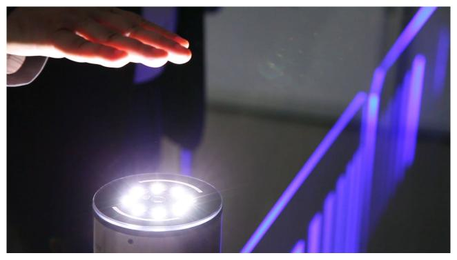
Figure: contactless fingerprints scanner integrated in eGate
