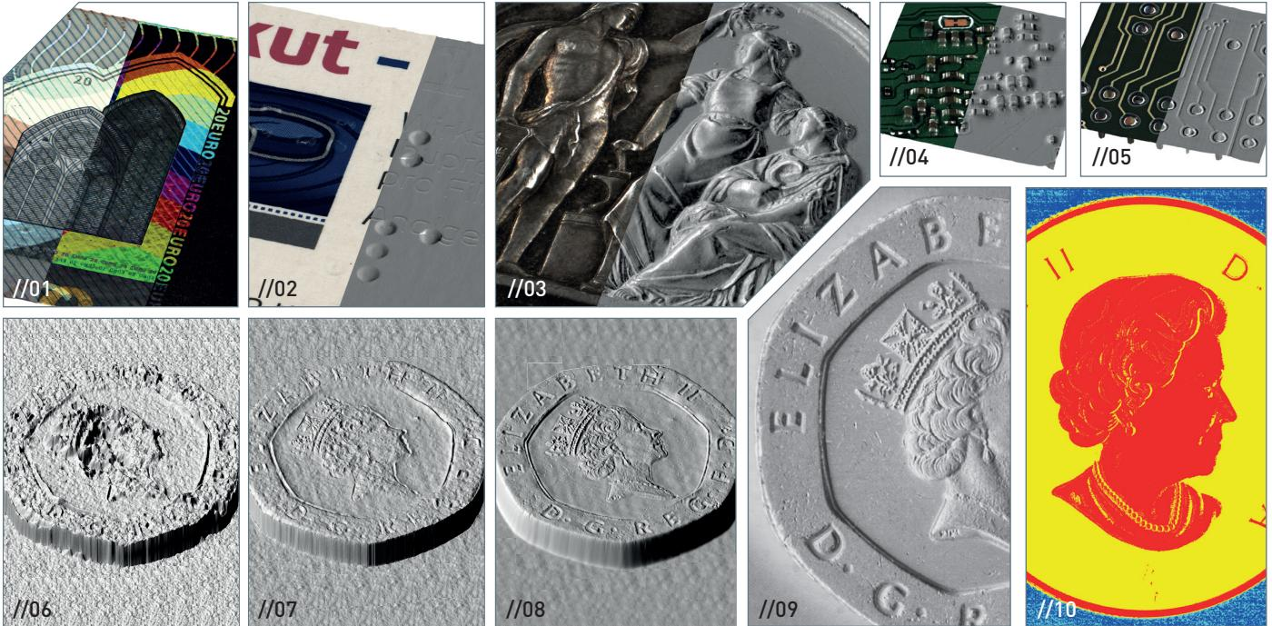
Instead of using several cameras or a microlens array on the sensor chip (reducing optical resolution), our inline computational imaging approach uses only one multi-linescan camera which simultaneously captures several object views exploiting the relative motion between camera and object. By high-performance computational processing of the light-field data it is possible, e.g. to derive depth information and obtain all-in-focus image with increased signal-to-noise ratio.
