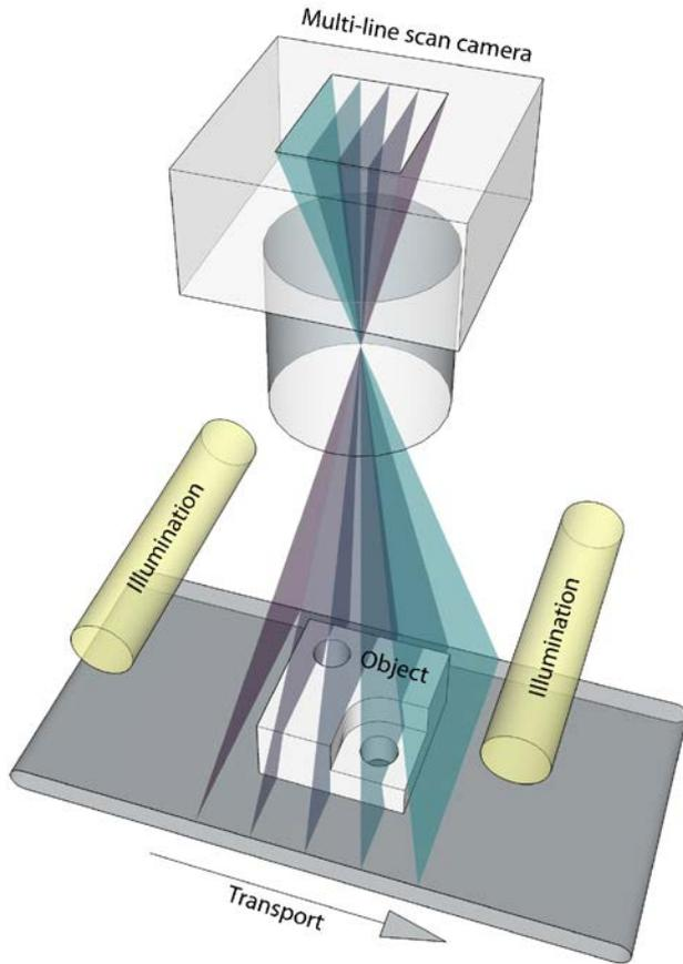
AIT ICI light field: Every view (image) is associated with a different viewing perspective (sensor line)
