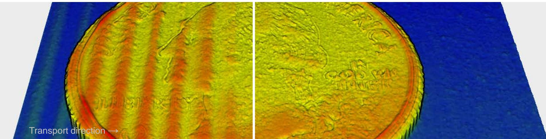
Depth ripples visible due to transport jitter
