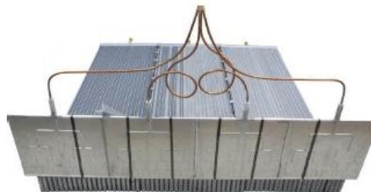
**b) all elements connected to the venturi distributor and evaporator core**
