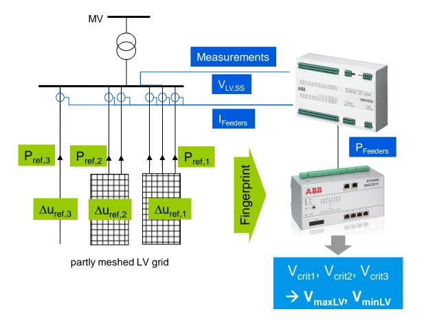
Estimation of critical voltages in the LV grid without extensive ICT
