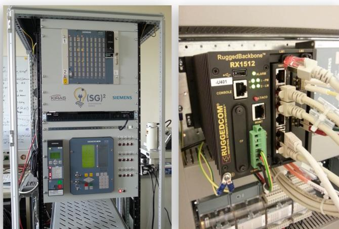
Fig. 3: Substation test system
