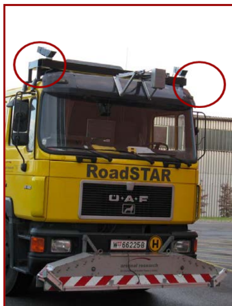
Figure 11: Position of stereoscopic video camera system on survey vehicle
