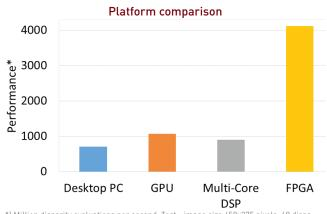
\*) Million disparity evaluations per second. Test - image size 450x375 pixels, 60 disparities. Desktop PC: Intel i7 with 4x2 Cores and 3GHz; GPU: GTX280 with 240 Cores and 1.3GHz; Multi-Core DSP: TMS320C6678 with 8 Cores and 1GHz; FPGA: XC7Z020 with 150MHz.
