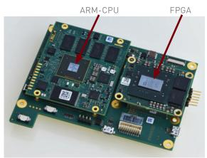
FPGA calculates high quality depth images in real-time
