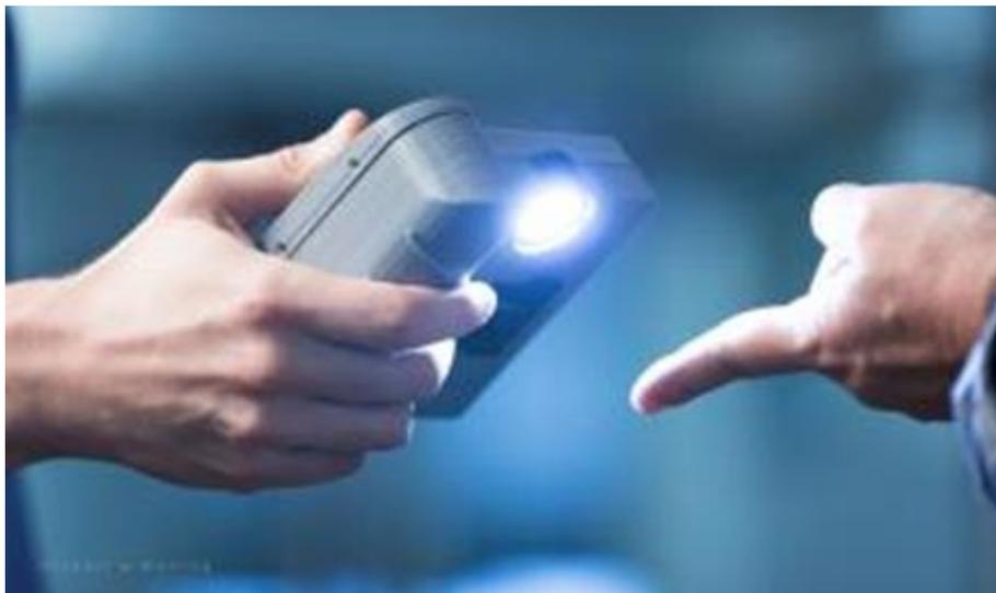
*Figure 4. Demonstrator of contactless and mobile fingerprint verification, source: AIT – European FP7 project MobilePass, [www.MobilePass-project.eu](http://www.MobilePass-project.eu)*
